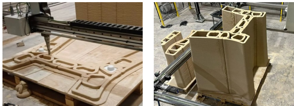
Figure 14 Printing procedure of the segments
