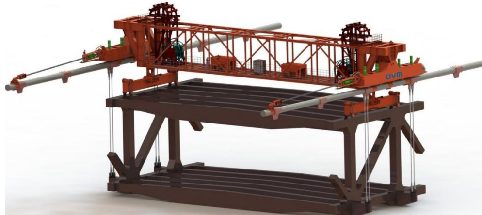
Figure 1 Structural assembly of cable-mounted cranes
