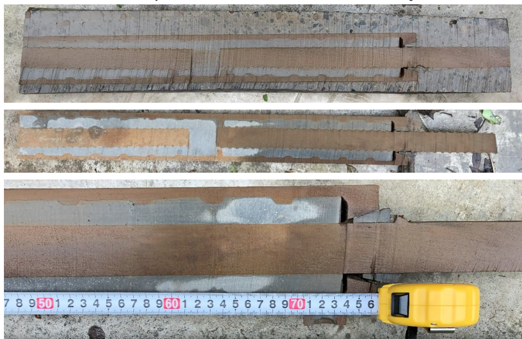
Figure 6 Example of a sectioned grouted sleeve—void near the grout outlet causing slightly reduced reinforcement anchorage length
