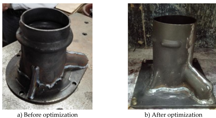
Figure 11 Structural optimization of the bearing plates
