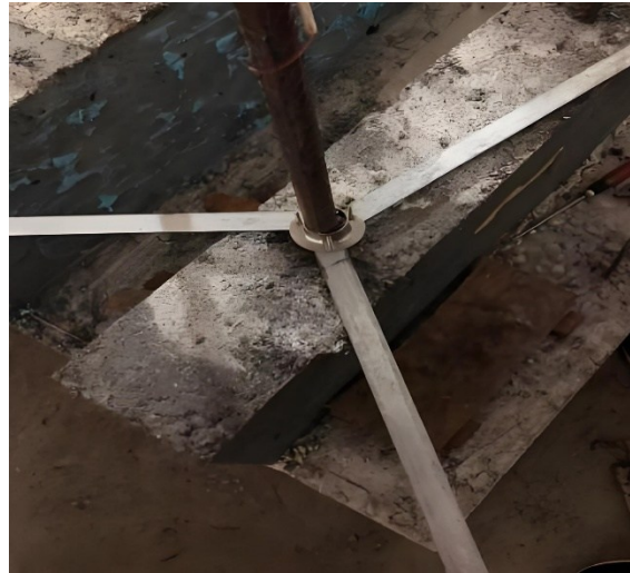
Figure 6 Fixed bracket for displacement sensors
