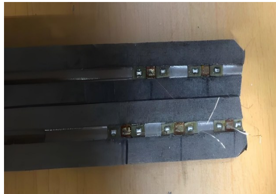
Figure 3 Strain gauges attached to the inside of the steel bars
