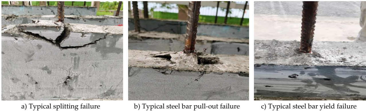
Figure 7 Sample failure mode
