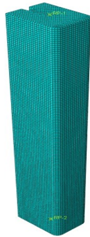
Figure 3 Concrete/ECC/UHPC/FRP mesh diagram
