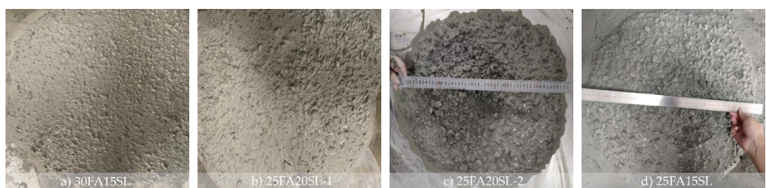
Figure 1 Workability of concrete with different mineral admixture ratios
