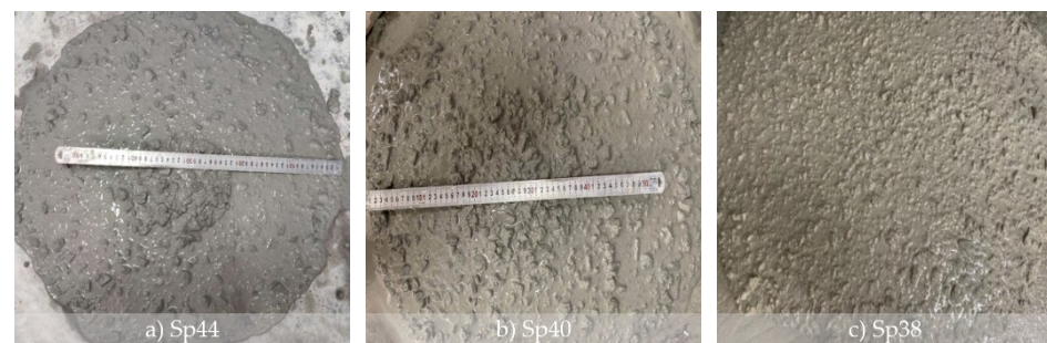
Figure 2 Workability of concrete with different sand ratios
