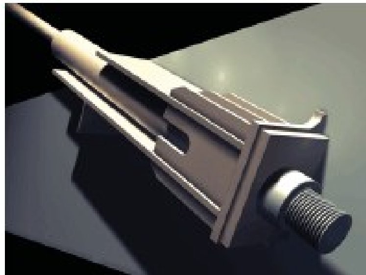
Figure 13 Example diagram of a steel anchor box on a beam
