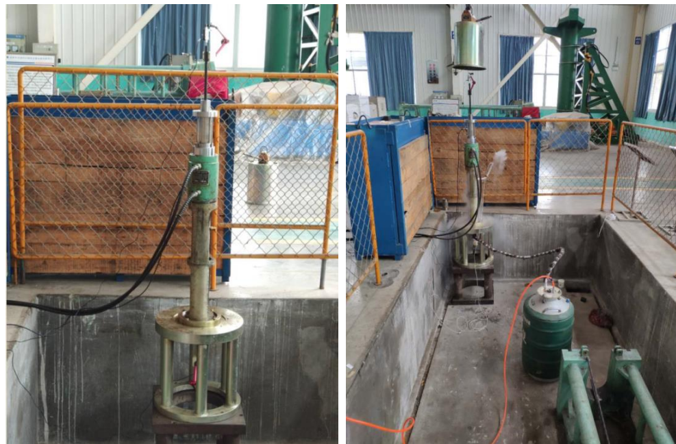
Figure 24 Slip test of the steel strand central wire in a cryogenic environment
