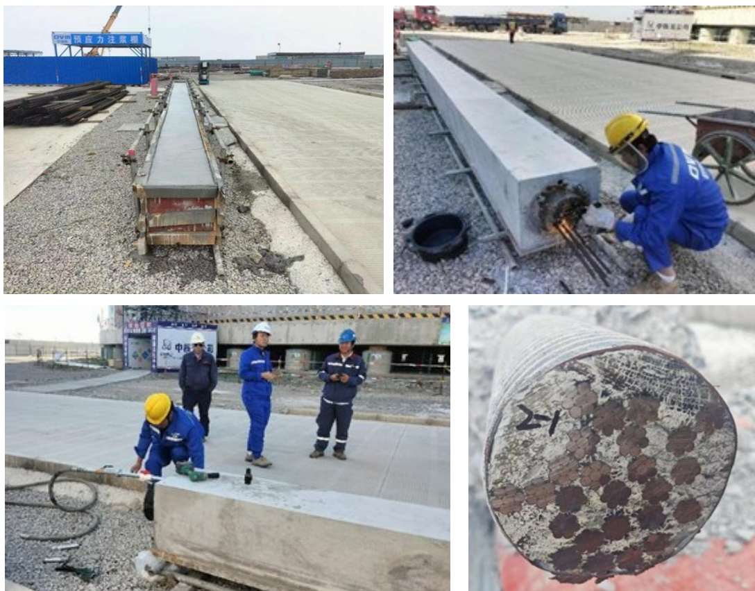
Figure 26 Full-scale grouting test in a prestressed duct
