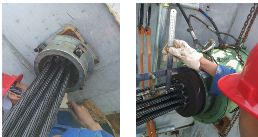
Figure 27 Friction test in the prestressed duct
