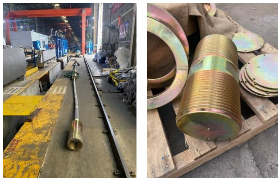
Figure 10 Main cable strand, connecting shaft and the end of the finished cable specimen
