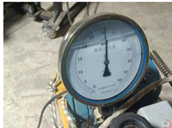
Figure 19 Reading hydraulic pressure gauge
