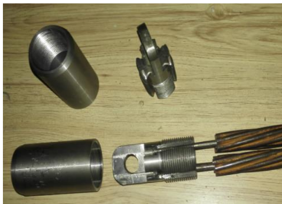
Figure 7 Fixing steel strand at pulling head
