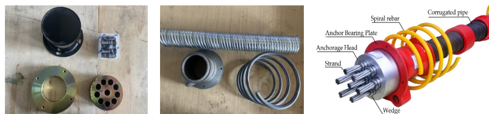
Figure 1 Diagram of a prestressed component
