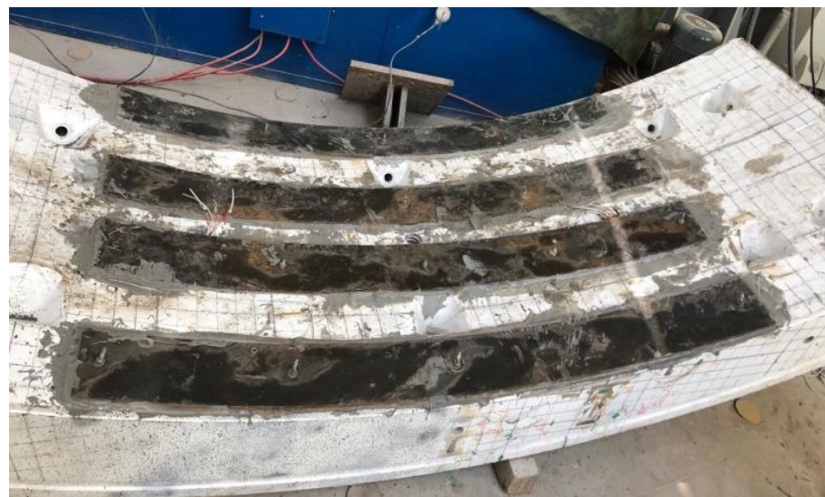
Figure 3 Steel plate reinforcement diagram
