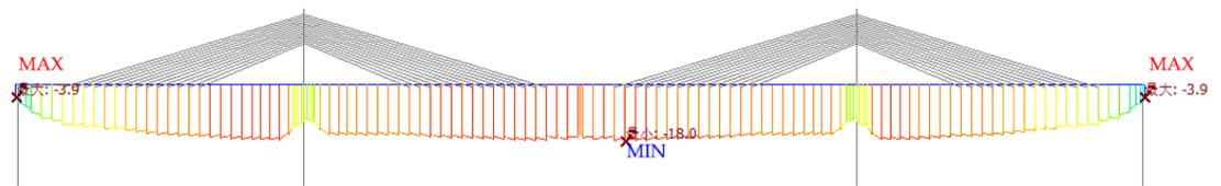
**Figure 15** Top-edge Stress Envelope Diagram of the Girder (Unit: MPa)
