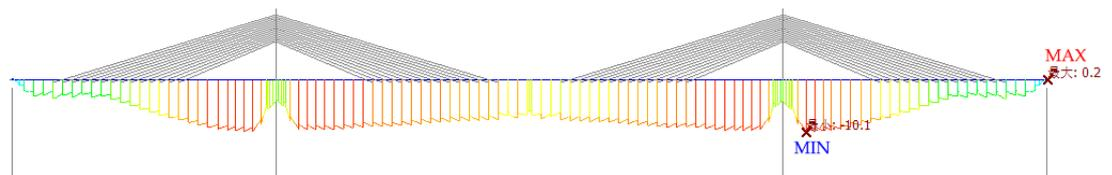
**Figure 13** Top-edge Stress Envelope Diagram of the Girder (Unit: MPa)
