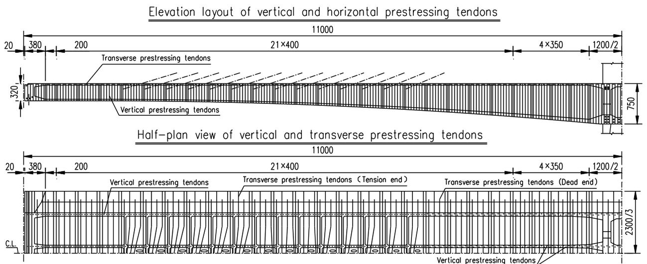
Figure 4 Layout Diagram of Transverse and Longitudinal Prestressed Tendons in the Girder (Side Span) (Unit: cm)
