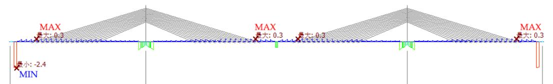
Figure 9 Maximum Stress on Top Edge of the Girder (Unit: MPa)
