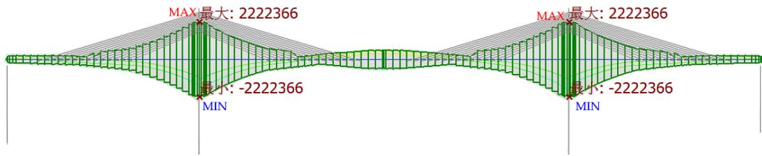
**Figure 11** Bending Torque Envelope of the Load-bearing Capacity of the Girder (Unit: N\*m)
