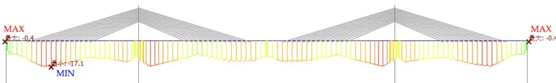
**Figure 16** Bottom-edge Stress Envelope Diagram of the Girder (Unit: MPa)
