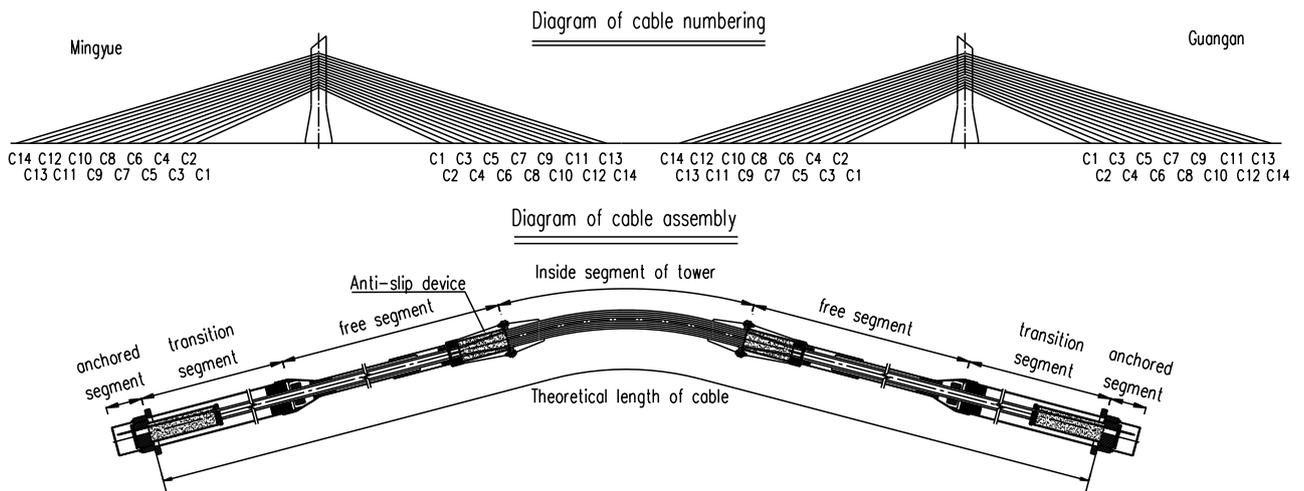
Figure 6 General Construction of Cables
