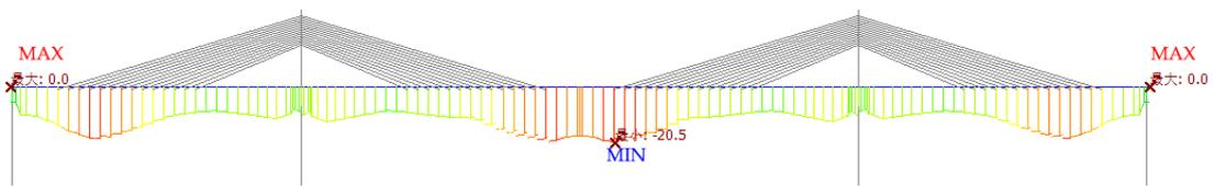
Figure 8 Minimum Stress on Bottom Edge of the Girder (Unit: MPa)
