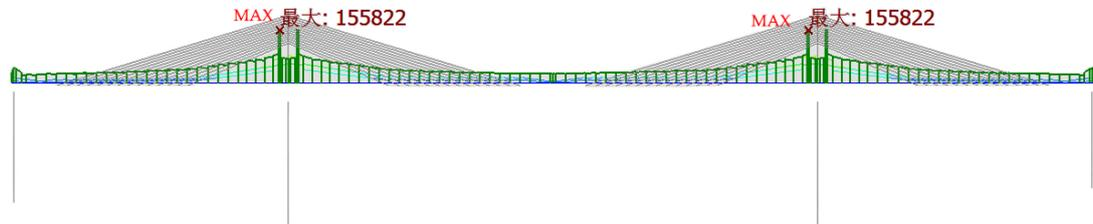
**Figure 12** Shear Envelope of the Load-bearing Capacity of the Girder (Unit: kN)
