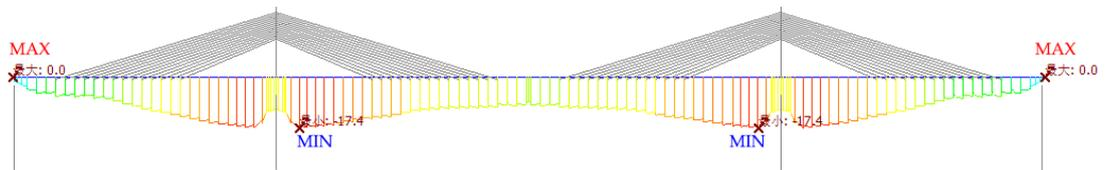
Figure 7 Minimum Stress on Top Edge of the Girder (Unit: MPa)
