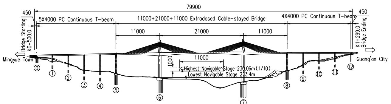
**Figure 1** Elevation View of the Mingyue Qujiang River Bridge in Guang'an (Unit: cm)
