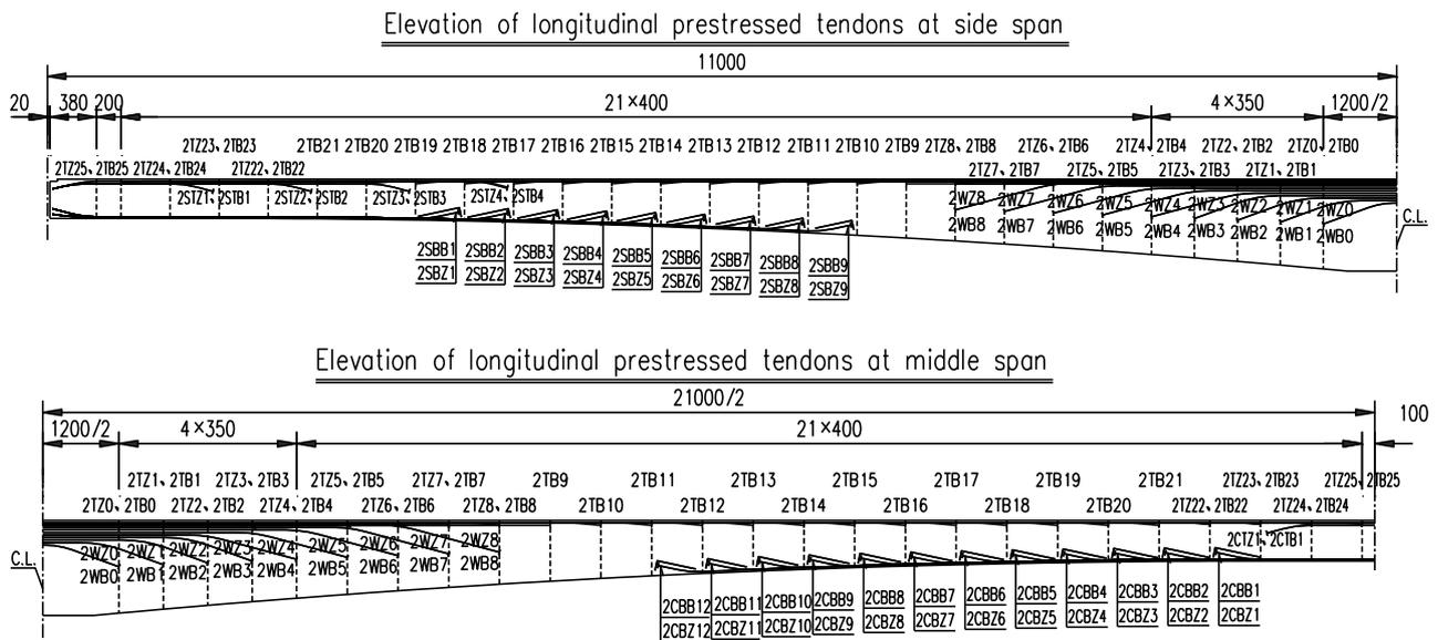
Figure 3 Layout Diagram of Longitudinal prestressed Tendons in the Girder (Unit: cm)
