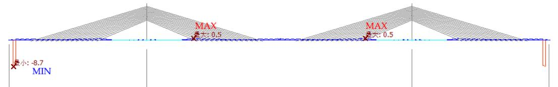
Figure 10 Maximum Stress on Bottom Edge of the Girder (Unit: MPa)
