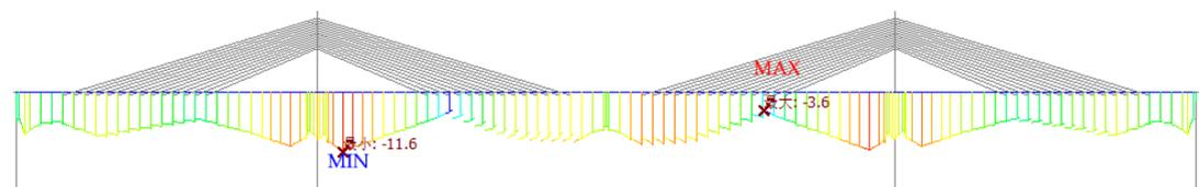
**Figure 14** Bottom-edge Stress Envelope Diagram of the Girder (Unit: MPa)
