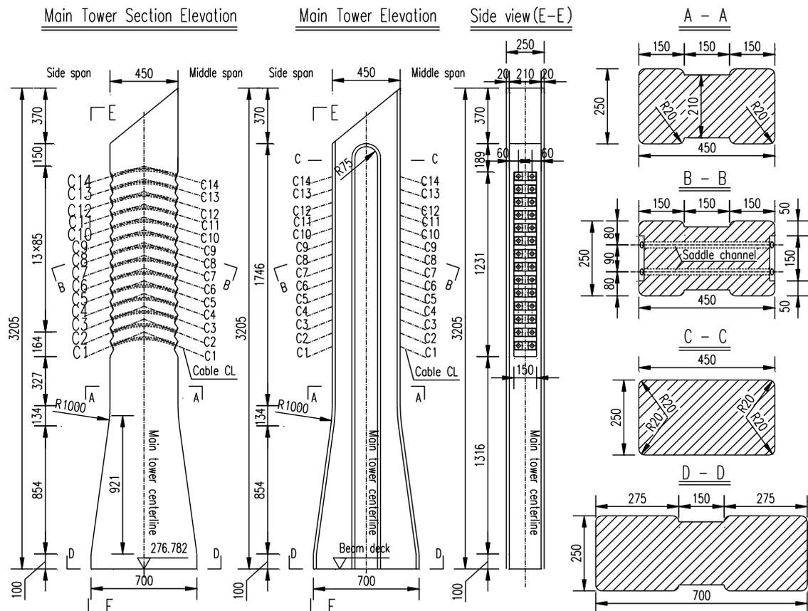
Figure 5 General Structure of the Main Tower (Unit: cm)
