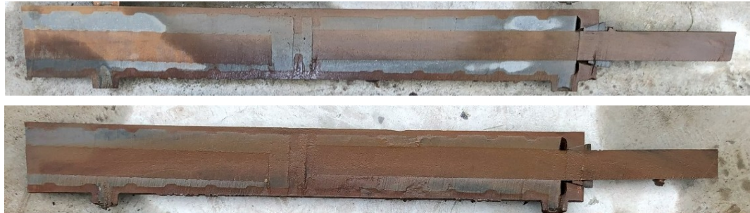
Figure 7 Example of a sectioned grouted sleeve—offset of embedded reinforcement bars in the pile cap
