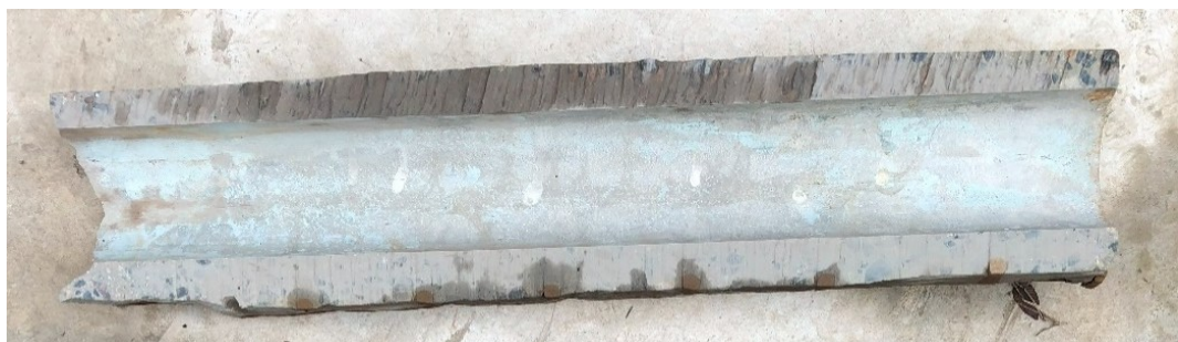
Figure 8 Example of a sectioned grouted sleeve—delamination between sleeve outer wall and concrete
