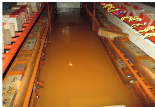
Figure 2 Seawater simulation test chamber
