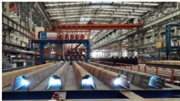
Figure 10 High-quality fully penetrated weld joints for U-ribs
