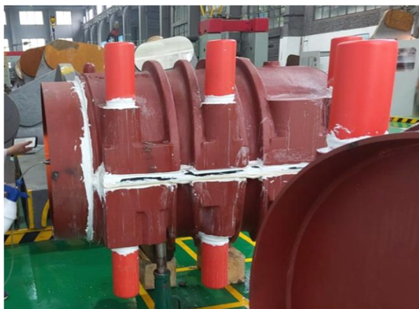
Figure 15 Triple-seal structure of the cable clamp
