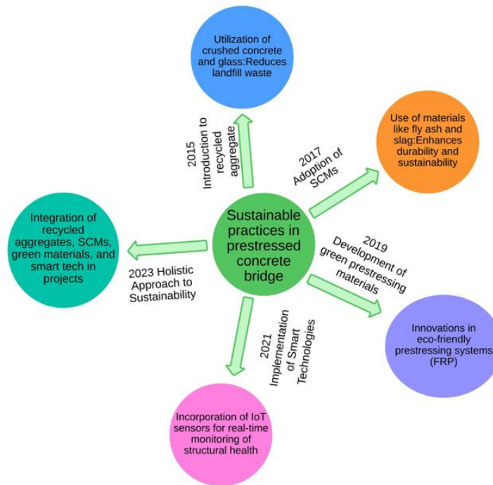
Figure 1 Evolution of sustainable practices in prestressed concrete bridge construction over the past decade.
